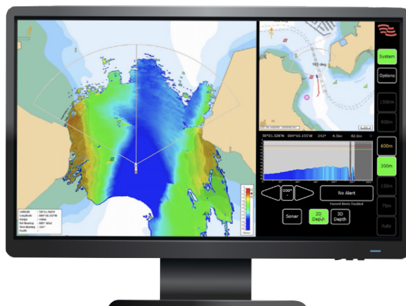
In 2D Mode Vigilant shows water depth colour coded on a bow up display. Good for confined waters where you want a detailed image around you.
