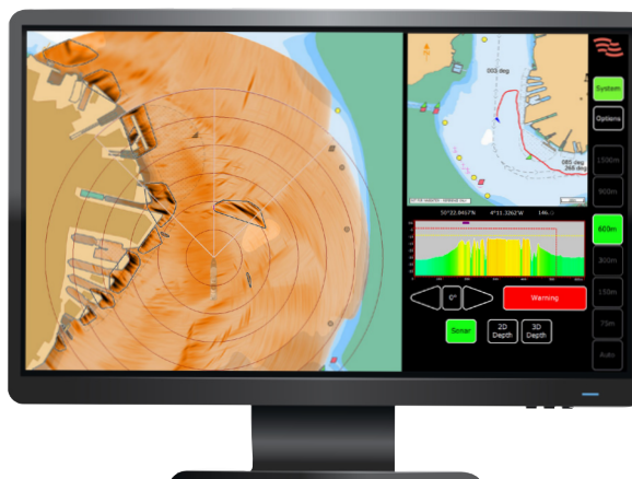
In Sonar mode Vigilant shows long range sonar echo intensities. Good for open water navigation to detect objects in the water.
