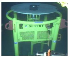
Sentry's 360° field of view provides a detection coverage radius of up to 1200 m, detecting leaks of monophase gas down to flow rates of 0.1 litre per minute, which is the equivalent of around one barrel of oil per day. For monophase oil, it detects up to one litre per minute, the equivalent of ten barrels of oil per day.
